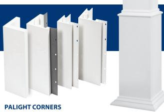
Palight Corners are designed with appearance in mind. Standard corners are available in 5/4" x 4" and 6" and are ideal for fiber cement board applications. Corners with J-channels and nailing fins are available in two sizes:  $3\frac{1}{2}$ " and  $5\frac{1}{2}$ ". The  $5\frac{1}{2}$ " size is also available with no J-channel and hinged nailing fins.
